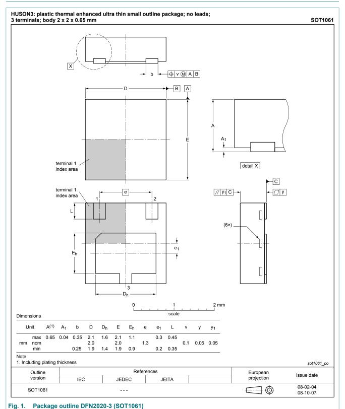
plastic, leadless thermal enhanced ultra thin small outline package; 3 terminals; 1.3 mm pitch; 2 mm x 2 mm x 0.65 mm body
