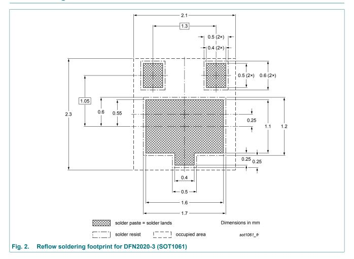
plastic, leadless thermal enhanced ultra thin small outline package; 3 terminals; 1.3 mm pitch; 2 mm x 2 mm x 0.65 mm body
